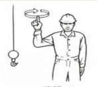
HOIST With forearm vertical, forefinger pointing up, move hand in small horizontal circles.
