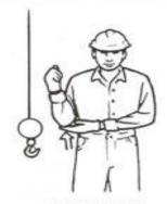
USE WHIPLINE (Auxiliary hoist) Tap elbow with one hand, then use regular signals.
